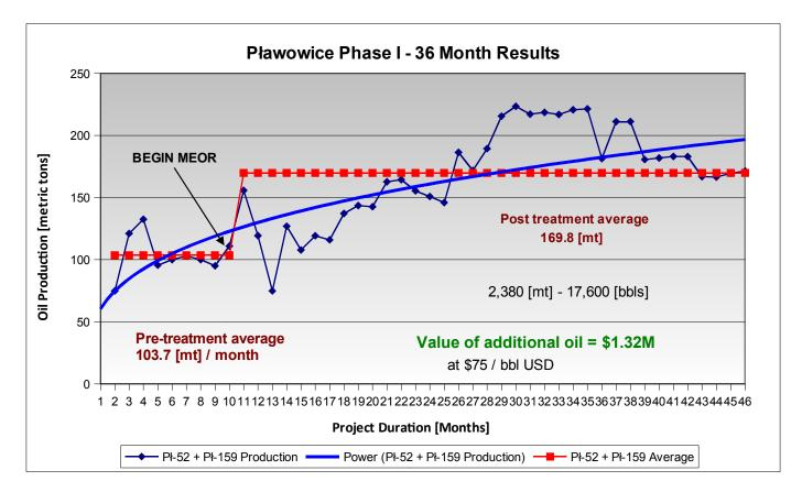
The spike in production following microbial system [MS] injection is attributed to biosurfactants produced during final grow-up of the MS slug ( $\pm$  20 mt) which took place at the Plawowice oil field. Injector problems account for the subsequent downturn. Production then trends sharply upwards once the injected MS becomes established in the formation and begins migrating towards the production
