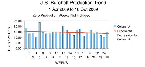
J. S. Burchett oil production trended downward slightly from 4/01/2009 up to the initial MEOR treatment on 10/16/2009 as indicated by the chart above. Production from 1/01/2009 through 10/16/2009 (235 production days) averaged = 1.89 BOPD, virtual identical to the 18 week (126 day) pre-treatment average of 1.90 BOPD
